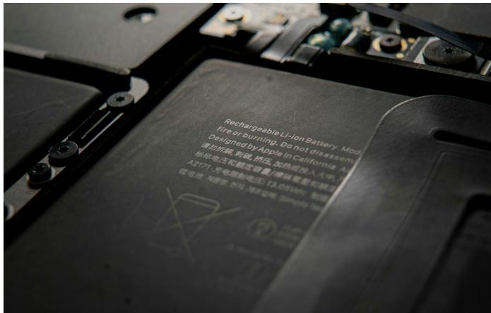
Thermal runaway can be caused by over or undercharging, manufacturing defects and mechanical abuse such as overheating or dropping your device.
