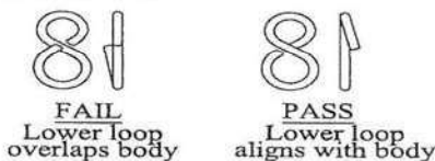
FIG. A1.18 Requirements for Fastening Devices Reference Paragraphs 6.4.5 and 6.4.5.1
